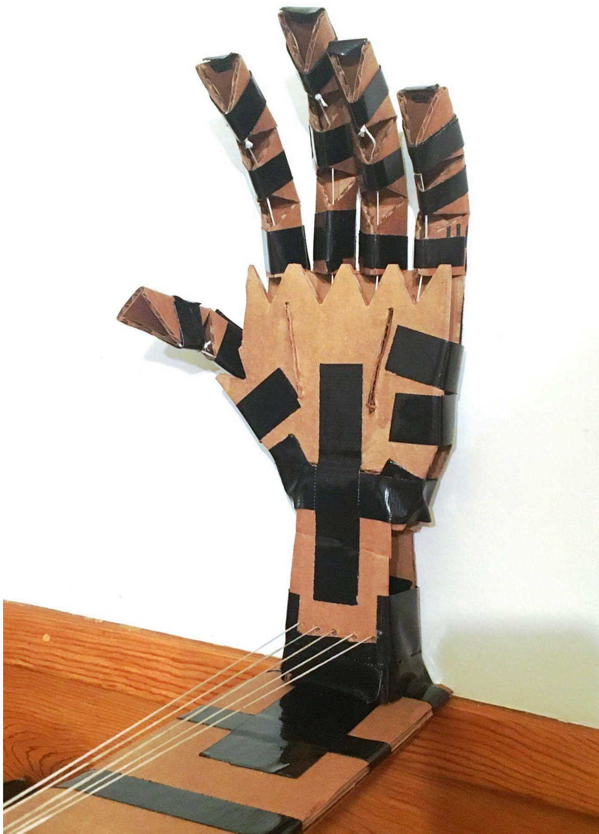
Mechanical design proof of concept prototype: cardboard, duct tape, and string.
